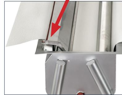
*In operation mode, the water skimming flap lies on the tissue or fleece web. Now the adjusting screw can be used to make individual settings. This can, for example, be helpful in the following cases:*
