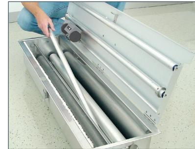
*When disassembling the device, the legs are pulled out of the lateral holders. The tubes of the frame are placed in the steep bath for transport. The folded lid is fixed in place using locking hooks.*
