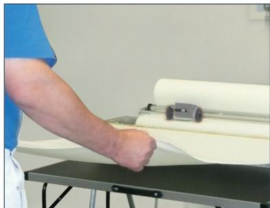
*The webs are drawn through the machine in the required lengths and are placed together in loops.*
