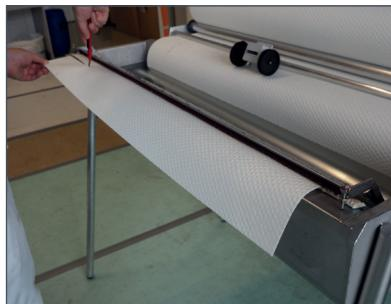
*The web is cut off on the cutting edge on the front of the steep bath. Only once the last web is run through it is cut off directly in front of the meter counter.*
